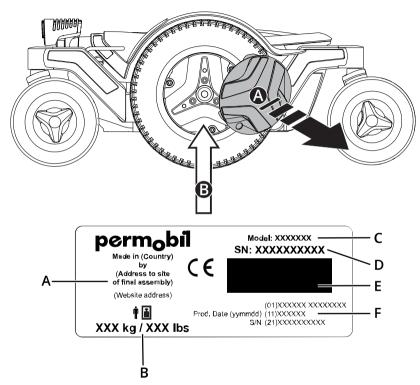
The serial number label is located on the lower, left hand side of the wheelchair chassis. Remove the rim  $\textcircled{\begin{tmatrix} \bullet \end{tmatrix}}$  for access to the serial number label  $\textcircled{\begin{tmatrix} \bullet \end{tmatrix}}$ .
