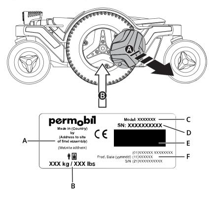
The serial number label is located on the lower, left hand side of the wheelchair chassis. Remove the rim **a** for access to the serial number label **b**.
