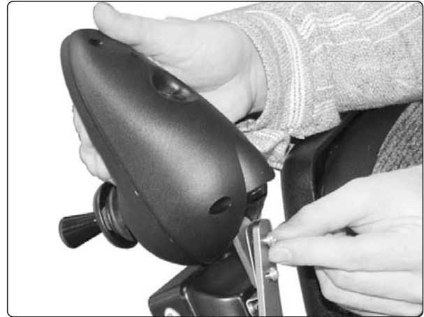
Fig. 48. The Control panel and Seat control panel bracket.
