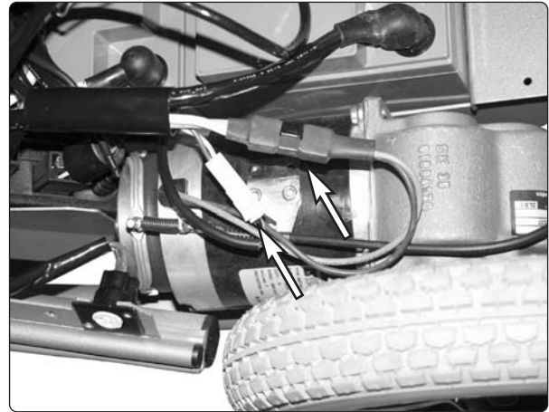
Fig. 19. The magnetic brake and drive motor electrical connectors.
