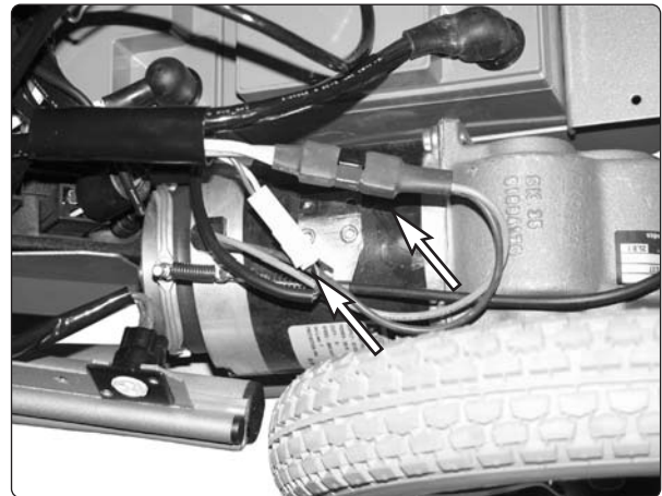
Fig. 31. Disconnect the electrical connectors.
