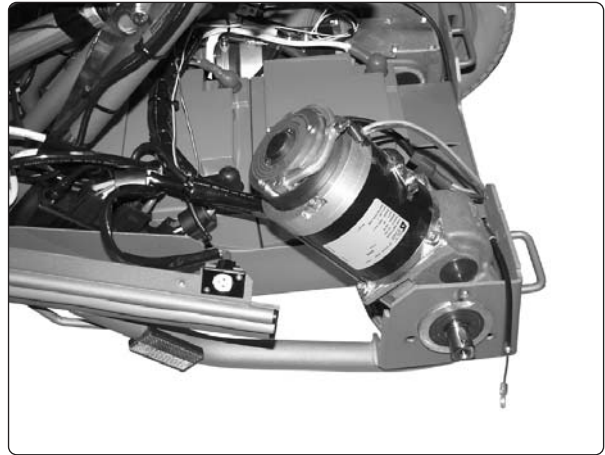
Fig. 22. Lifting up the rear end of the motor makes the magnetic brake more accessible.
