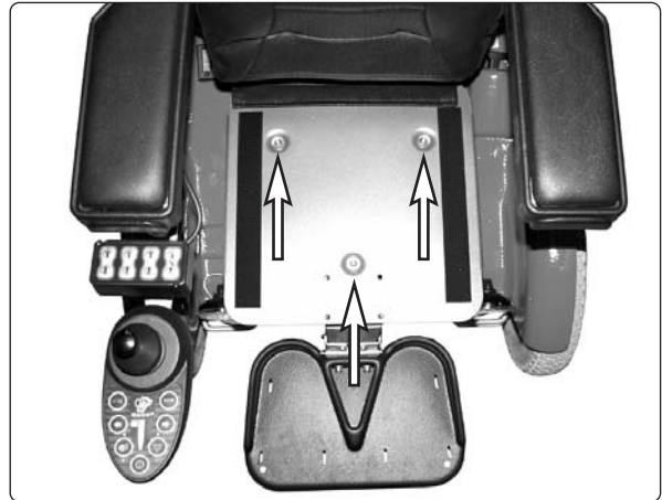
Fig. 35. The seat plate is attached by three bolts.
