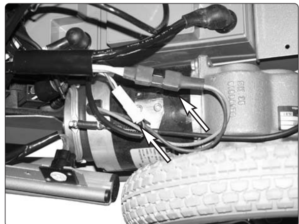
Fig. 29. Magnetic brake and drive motor electrical connectors.
