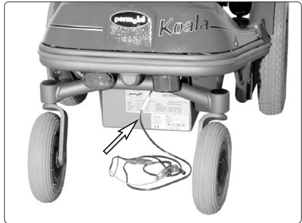
Fig. 4. Connecting the cable for emergency operation.
