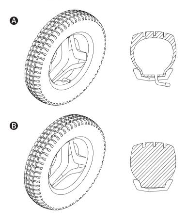
The wheelchair drive wheels have pneumatic tires or flat-free (foam filled) tires. The caster wheels have pneumatic tires or solid polyurethane tires.
