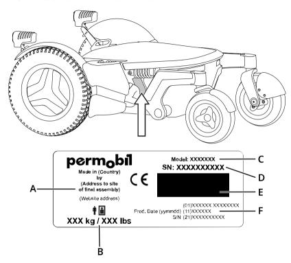
The serial number label is located on the lower, left hand side of the wheelchair chassis. Look to the right of the drive wheel.
