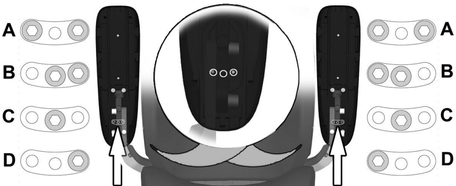
The endpoints are set by moving one or two screws between three different positions underneath the armrest.
