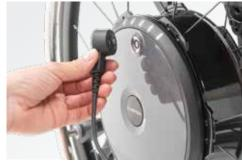
Everything under control: On/Off switch with magnetic EasyConnex charging socket. The plug of the e-motion battery charger automatically finds its position.
