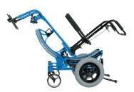
Tilt arcs telescope minimising frame length.
