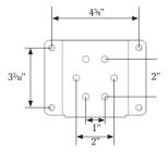
Detachable Mount to Hole Spacing Conversion Plate M2010
