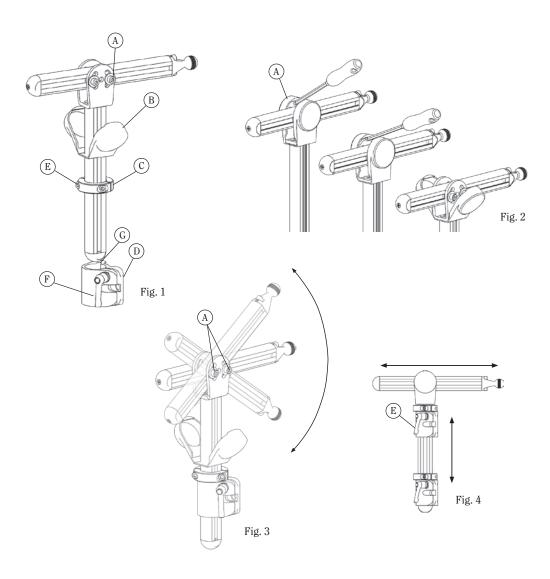
All Whitmyer Head Support rotational mounting balls are manufactured with a machined knurl pattern. When the collar is tightened, the specialized hardened knurls bite into the radius to eliminate unwanted movement.
