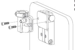
Note: Replace knob with  $\frac{1}{4}$ "-20 x  $\frac{3}{4}$ " bolt (MW010210) to disable detach function.
