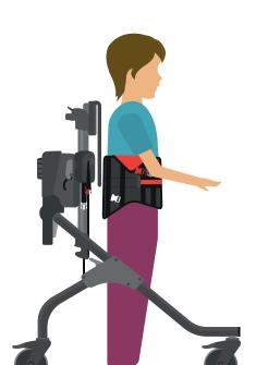
Transfer the child from the frame from standing or hoisted position by opening the white, red and grey buckles to release the harness from the frame. Alternatively open the grey buckles, groin straps and wrap, and assist the child to step out from the harness.
