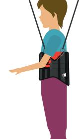
Hoisting: Attach one hoisting strap per side, with an end attached to the front and rear hoist attachment loops. Position the child's arms inside the loops to maintain comfort during the transfer.
