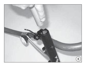
**Risk of injury as a result of incorrectly mounted grip bar.** The maximum height setting of the grip bar is predetermined by an extension limit. Adjustments beyond this range are not permitted.
