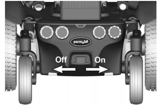
Figure 69. Resetting the main fuse
