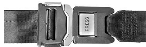
Figure 42. Belt buckle locked properly in the snap lock.
