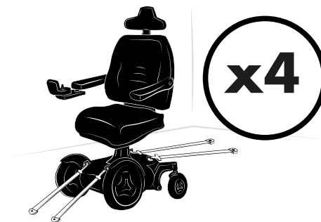
Figure 56. The wheelchair has four tie-down points. The wheelchair and tie-down position in this picture is generic.
