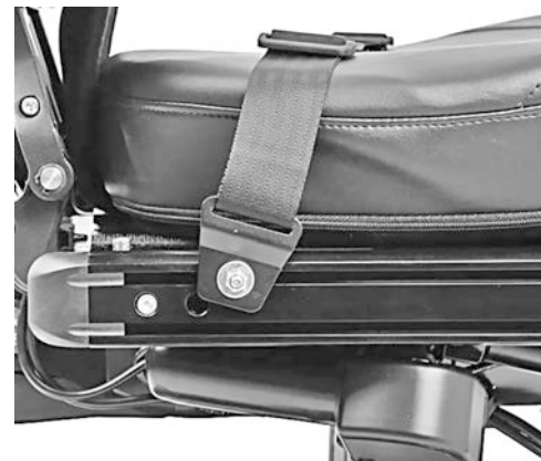
Figure 41. Attaching the positioning belt
