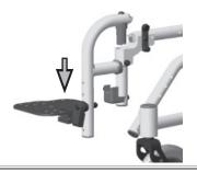
To attach the hanger, line up the pivot saddle with it's receiver on the frame and insert downward pressure until hanger locks into place.
