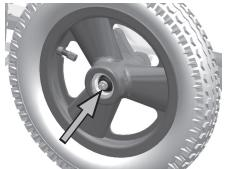
Disengage wheel lock, push the quick release axle button and pull wheel off of the frame.
