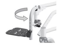
Pull outward on the lever (away from the chair). This will enable the hanger to swing away for ease of transfer.
