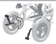
5. Rotate the anti-tip tubes upward as shown until they "click" into place.
