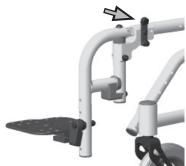
Pull back on the lever towards the chair. This will enable the hanger to pop-up and swing away for ease of transfer.
