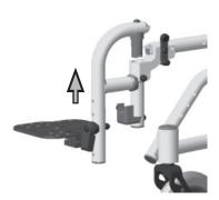
To remove the hanger, lift the hanger upward until the pivot saddle is out of it's receiver on the frame.
