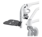
To attach the hanger, insert the pivot bushing into the frame receiver tube, at an angle as shown. Rotate the hanger inward until the latch snaps into place.
