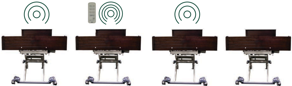
In pairing mode, the light/sound frequency will increase when the HB200 gets closer to a control box.
