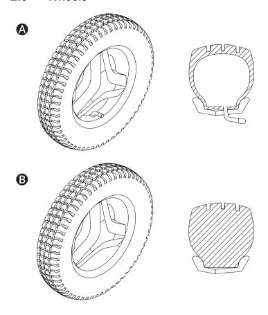
The wheelchair drive wheels have pneumatic tires or flat-free (foam filled) tires. The caster wheels have solid polyurethane tires.
