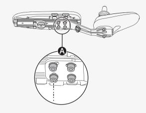
This is how you adjust the angle of the control panel.
