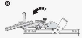
If your backrest does not have a manual quick release, do the procedure that follows to fold the backrest.
