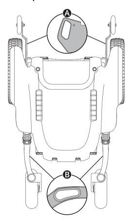
The wheelchair is equipped with four tie-down points used for transportation  $\rightleftharpoons$   $\overleftrightarrow{\bullet}$ . Two in the front  $\textcircled{\bullet}$  and two in the rear  $\textcircled{\bullet}$ .
