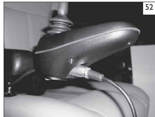
Off-board charger port located under joystick
