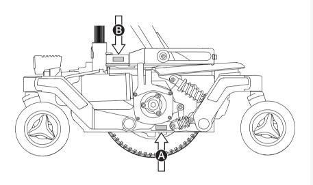
The serial number label is located on the lower, left side of the wheelchair chassis (4). An additional serial number label is located on the seat tilt (4). You may need to tilt the seat to see the serial number label.
