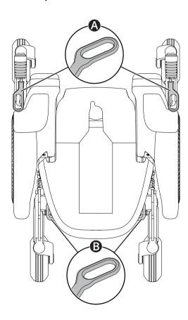
The wheelchair is equipped with four tie-down points used for transportation  $\rightleftharpoons$   $\overleftrightarrow{A}$   $\rightleftharpoons$ . Two in the front (A) and two in the rear (B).
