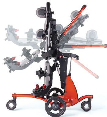
The Stander has 0°–90° gas-spring-assisted tilt adjustment.
