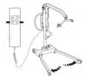
• The red emergency stop button, located on the rear of the control box, is in the OFF (out) position.
