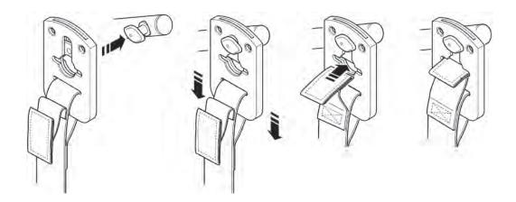
Securi3 sling attachment system. Example of installation.
