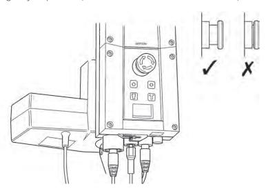
• Push the up and down buttons on the hand control and confirm the boom rises and lowers.
