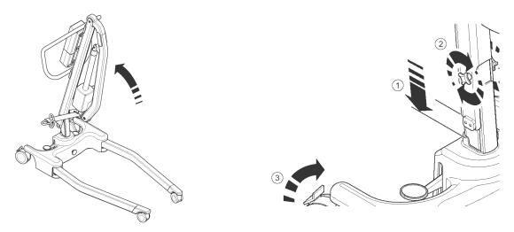
5. Open legs fully. ENSURE leg-locking knob inserts flush against the base casting and the legs will no longer move freely. The legs will then only operate by the use of the foot pedal mechanism located at the rear of the base.
